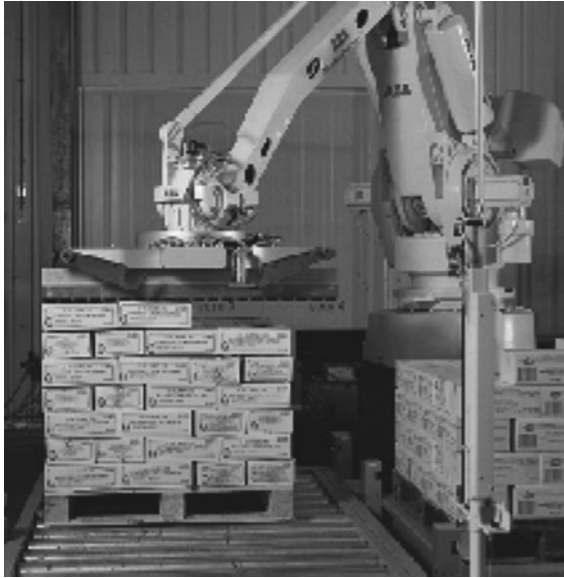
FIGURE 45.12 Palletizing robot application.
