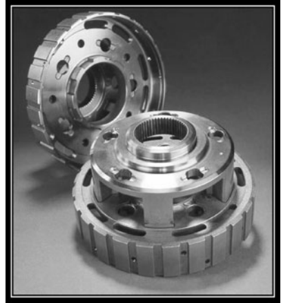
FIGURE 20.4 Copper infiltrated and furnace brazed three-piece planetary carrier for automotive transmission. (Courtesy of Metal Powder Industries Federation, Princeton, NJ.)
