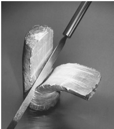
FIGURE 19.4 An aluminum billet is heated to the consistency of ice cream for use in the semisolid process.
