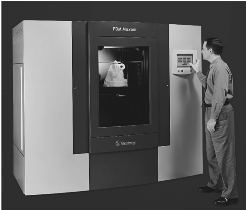
FIGURE 5.1 From small 3D printers to large format devices such as the FDM Maxum pictured here, rapid prototyping systems offer a wide range of functionality, price, and performance. (Photo courtesy of Stratasis, Inc.)
