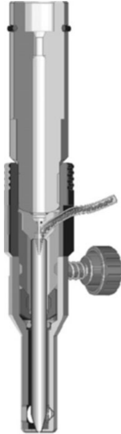
FIGURE 38.5 The architecture of an abrasive jet is fairly simple.
