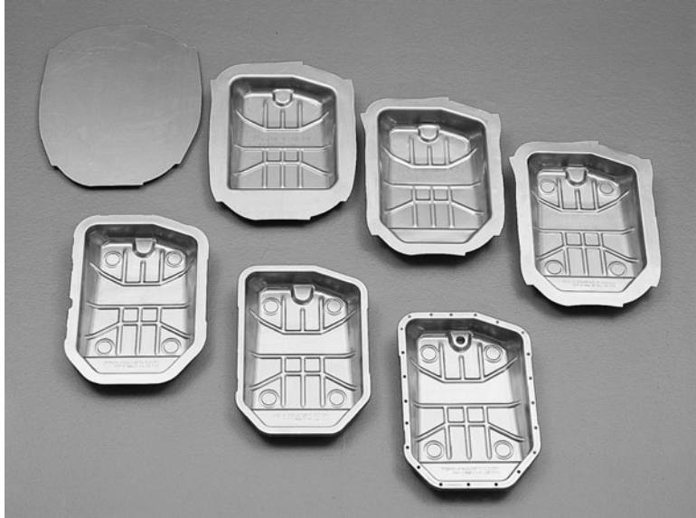
FIGURE 23.3 Line dies—production steps for the manufacture of an oil pan.
