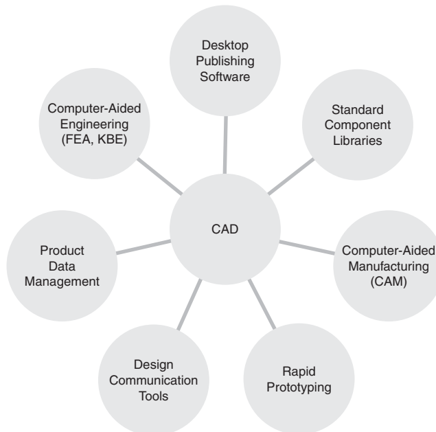
FIGURE 9.5 CAD data drives and interacts with a broad array of tools and technologies. (Courtesy of SolidWorks Corporation.)
