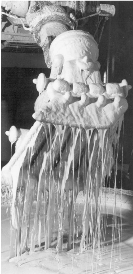
FIGURE 19.5 Investment casting, or the lost wax process, offers a high degree of precision in regard to dimensions as well as excellent surface finishes. This photograph shows covering the pattern assembly with a ceramic slurry to produce a monolithic mold.
