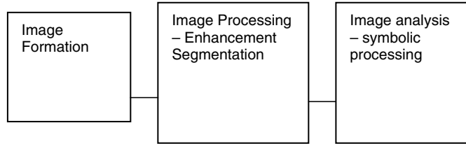
FIGURE 46.1 Machine vision block diagram.
