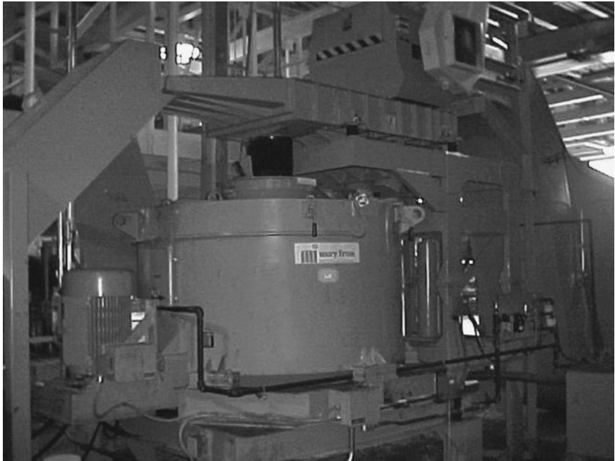
FIGURE 43.3 Heavy-duty wringers that have continuous feed systems are recommended for large volumes of chip processing. (Photo courtesy of Mayfran International.)
